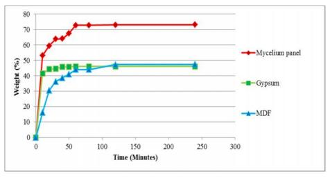
Figure 9: Water Absorption Percentage of Mycelium, Gypsum and MDF Panels.
