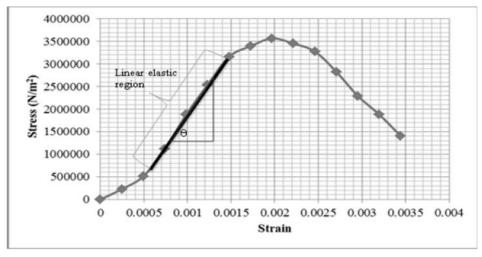
Figure 6: Stress-Stain Curve of Mycelium Panel
