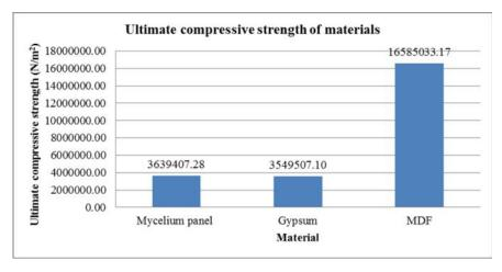
Figure 4: Ultimate Compressive Strength of Mycelium, Gypsum and MDF Panels
