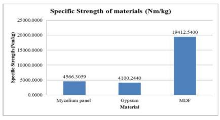
Figure 5: Specific Strength of Mycelium, Gypsum and MDF Panels
