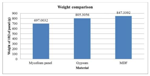
Figure 10: Weight of Mycelium, Gypsum and MDF Panels (1ft<sup>2</sup>)
