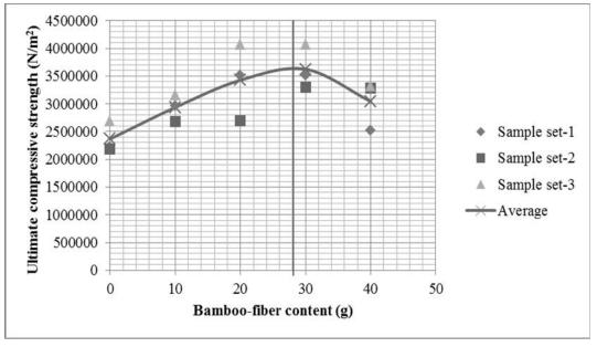
Figure 3: Ultimate Compressive Strength of Mycelium Panel Specimens
