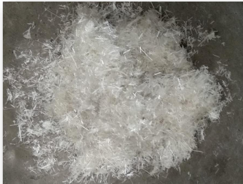
Figure 6.9: The glass fibers which were cut and prepared for mixing
