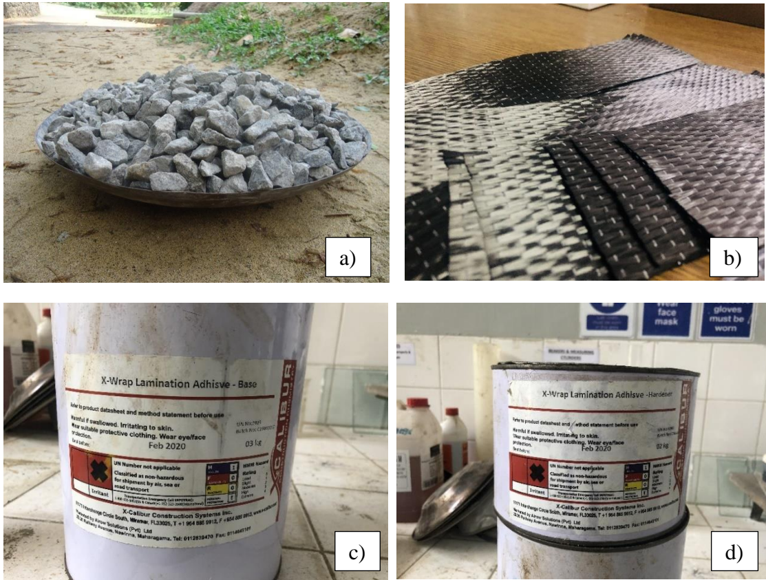
Figure 7-3 - a) Coarse aggregates b) CFRP fabric c) Adhesive - base d) Adhesive - Hardener
