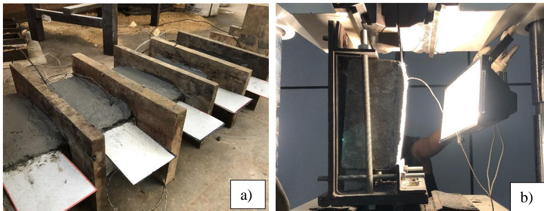
Figure 7-10 - a) Application of insulation layer b) Halogen lamps for elevating temperature
