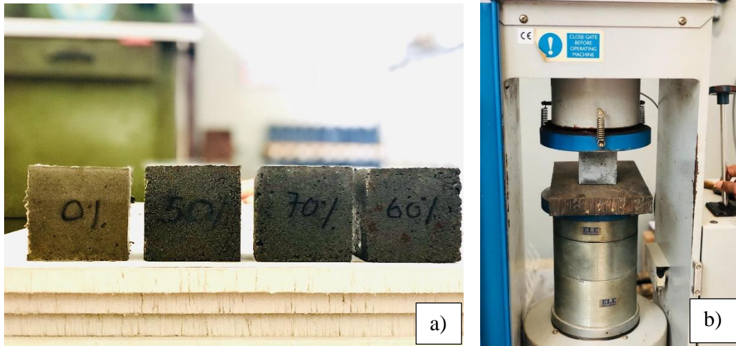
Figure 4-6 - a) Compressive strength test cubes b) Compressive strength testing
