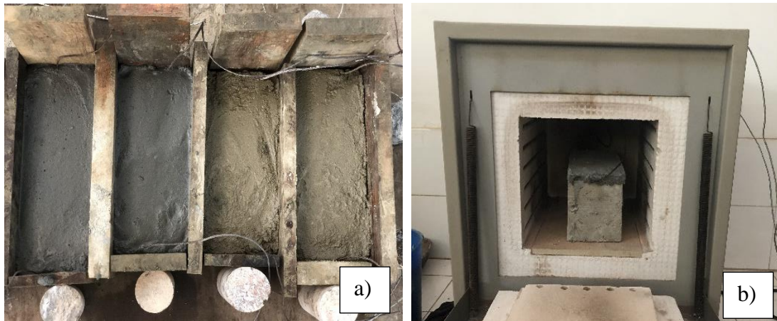
Figure 7-6 - a) Application of insulation layer b) Testing in Furnace
