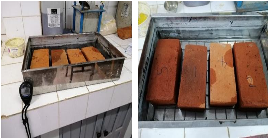
Figure 4. 3: Determination of initial rate of water absorption for FCB units
