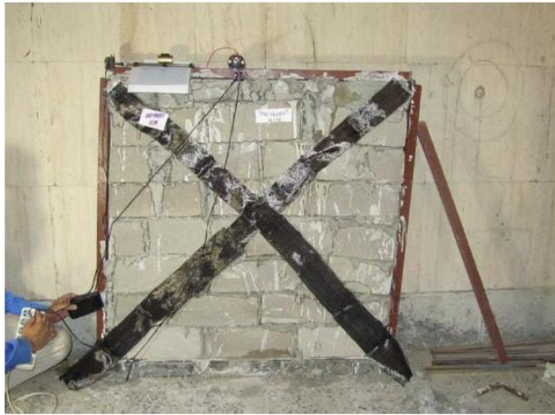
Figure 2. 9: Test apparatus with CFRP applied to wall
