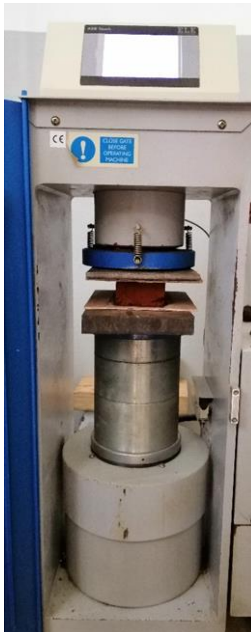
Figure 4. 2: Testing the compressive strength of masonry units
