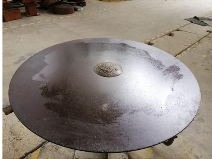
Figure 4. 6: Mortar after jolting for 15 seconds
