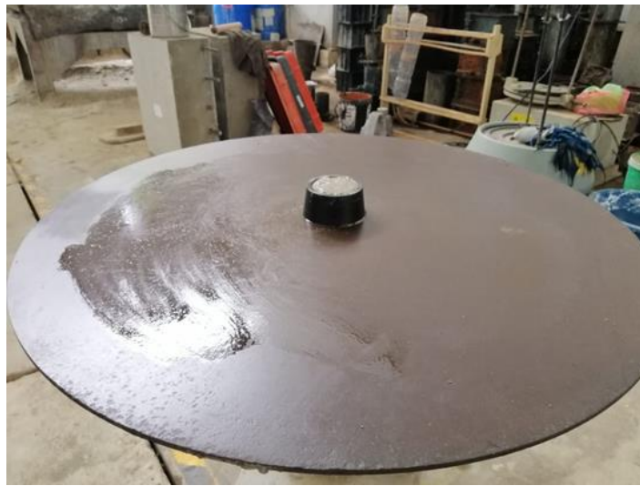
Figure 4. 4: Compacted mortar in the mold
