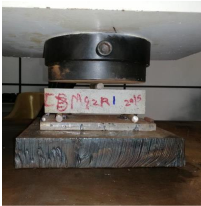
Figure 4. 7: Flexural Testing of a mortar prism
