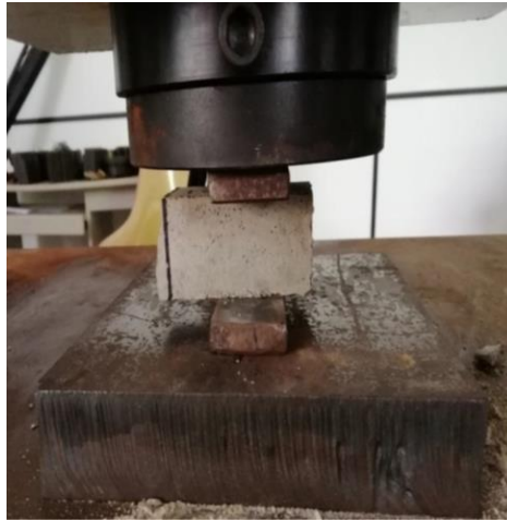
Figure 4. 8: Compression testing of a mortar prism
