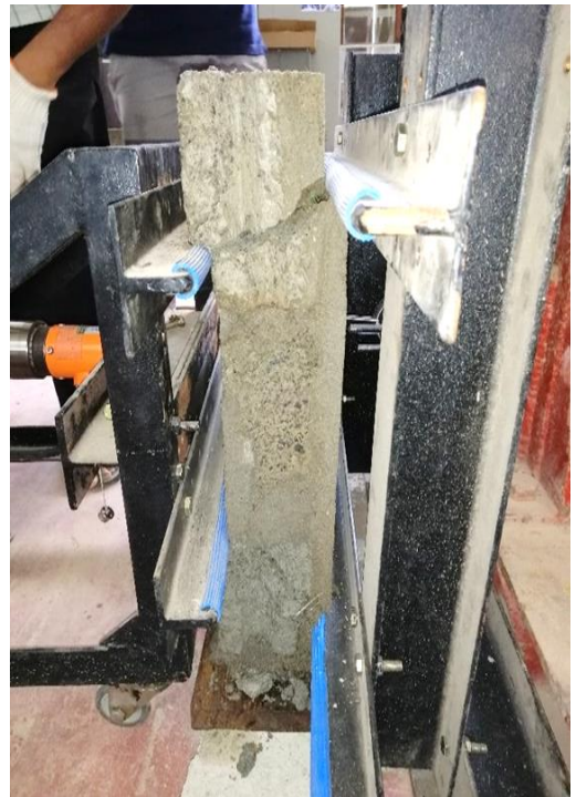
Crack in the masonry unit
