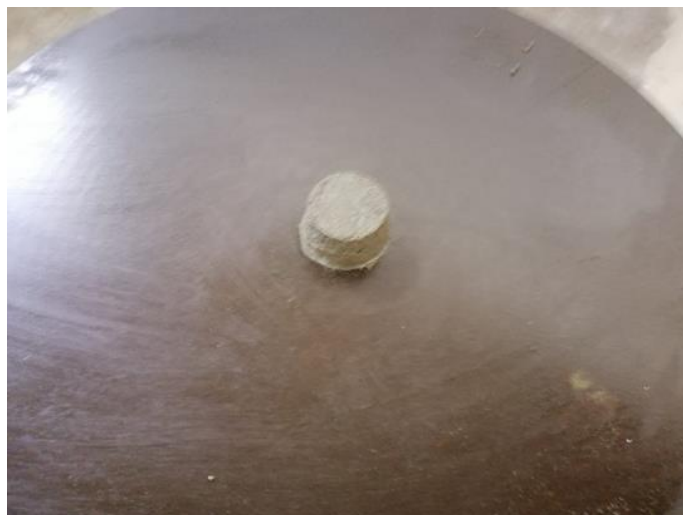
Figure 4. 5: Condition of the mortar after removing the mold
