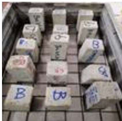
Figure 4. 9: Testing arrangement for water absorption coefficient of mortar prisms
