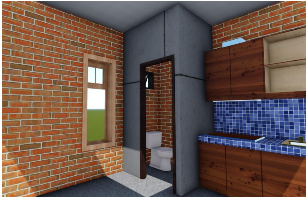
Figure 10: Lightweight Partition walls of the washroom to prevent the overloading of the first-floor slab
