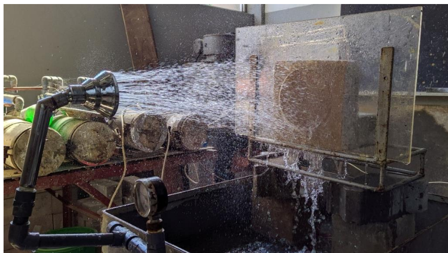
Figure 18: Erosion test on progress
