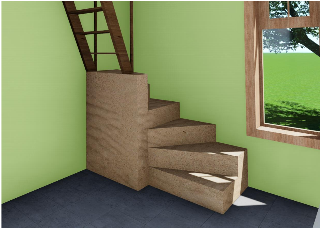
Figure 8: First few solid steps of the staircase out of CSRE
