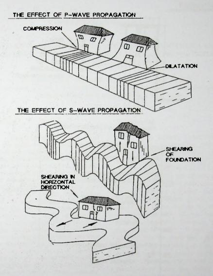
Figure 1: Effects of P and S waves on structural damage
