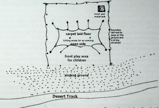
Figure 4: Layout of a solitary hut (open)
