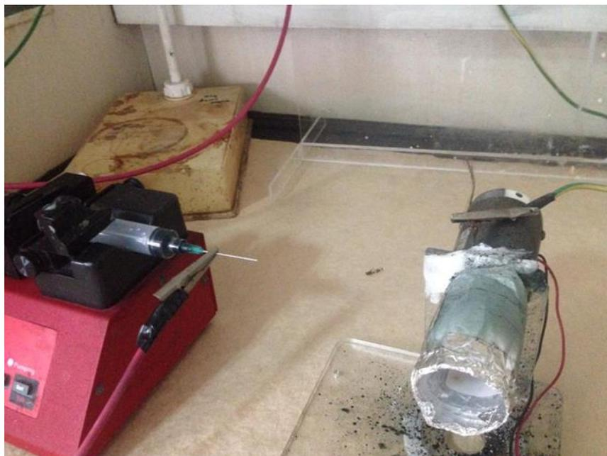
Figure 4.6: A photo of the electrospinning setup with rotational drum collector.
