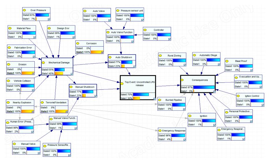
Figure 3.8: Application of the defined accident scenario to the Bayesian network
