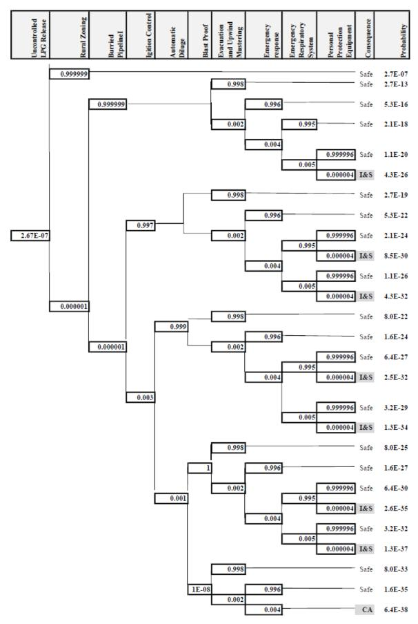
Figure 3.5: Event Tree diagram (i.e. Right portion of the Bow-Tie diagram)
