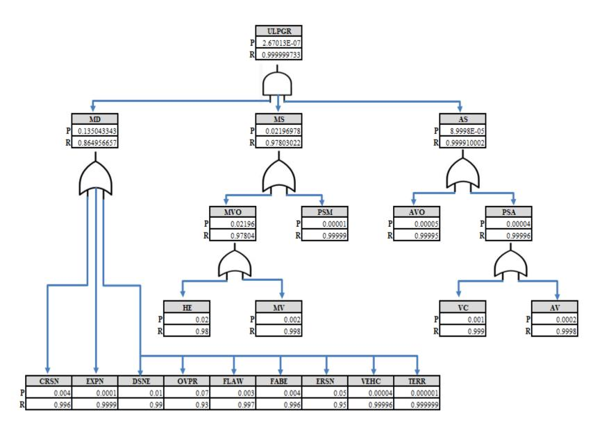
Figure 3.4: Fault Tree diagram (Left portion of the Bow-Tie diagram)
