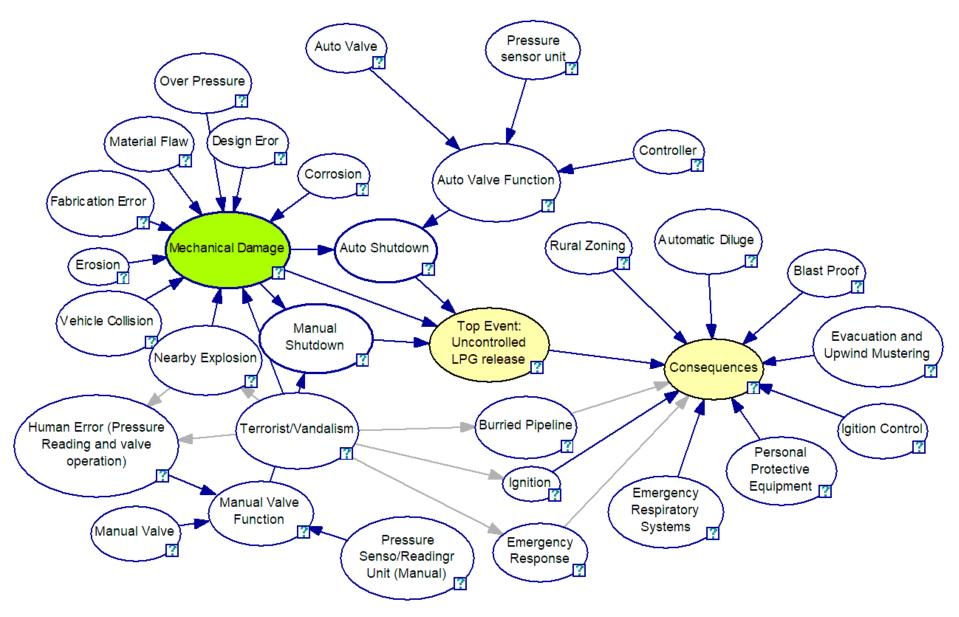
Figure 3.6: Bayesian network for the defined scenario Using GeNIe software
