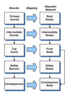
Figure 2.2: BT into BN Mapping algorithm [21]
