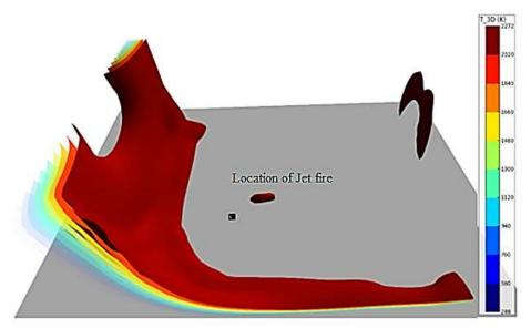
Figure 3.9: Surface diagram of the temperature distribution due to jet fire
