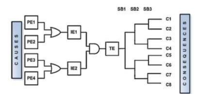
Figure 2.1: A Model Bow-Tie diagram [21]
