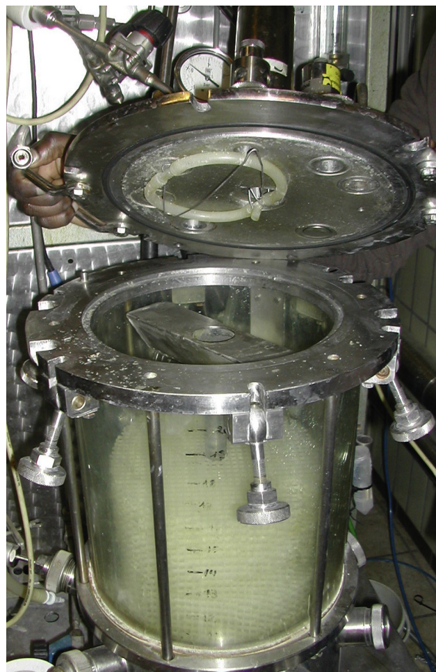
Fig. 1 – Lantec HD Q-PAC bed and rotating liquid distributor inside 20 L TBSBR.
