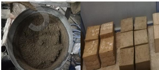
Figure 2: Soil mixture and cast blocks
