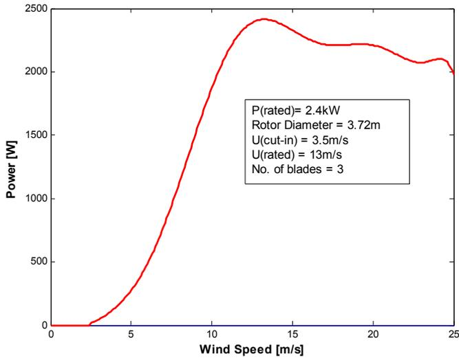
**Fig. 1.** Skystream 3.7 (Manufacturer) Power Curve including turbine operating characteristics.
