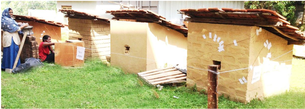
Figure 4: One-meter house models made to calibrate thermal conductivity coefficient
