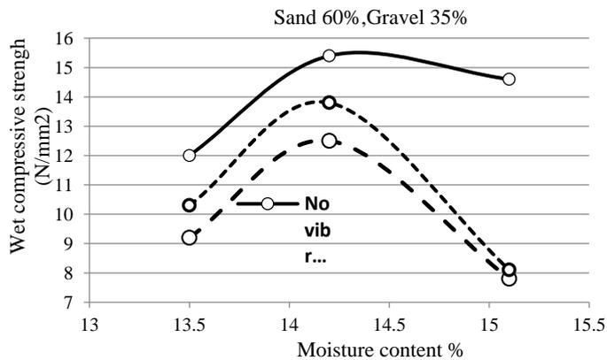
Figure 12: Variation of wet compressive strength with moisture content.
