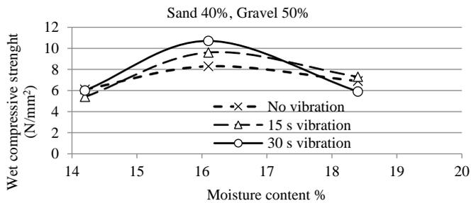
Figure 11: Variation of wet com. strength with sand 40% and gravel 50%
