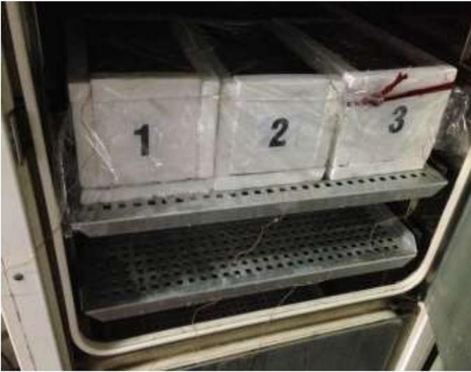
Figure 7: Freeze thaw cycle testing in climate chamber
