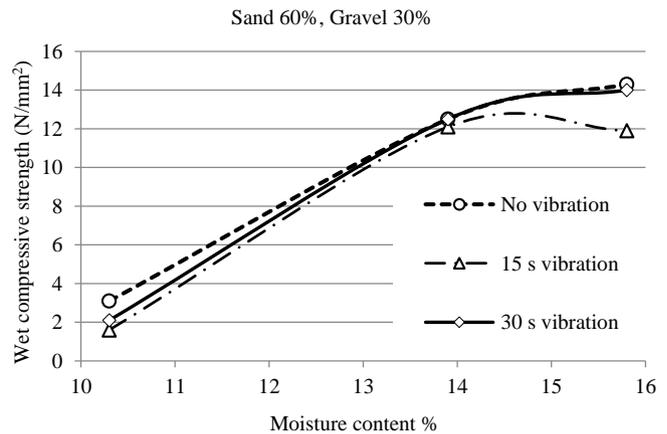
Figure 9: Variation of wet com. strength with sand 60% and gravel 30%
