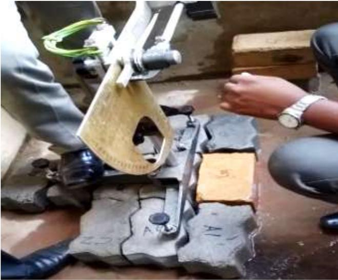
Figure 17: Skid resistance testing process
