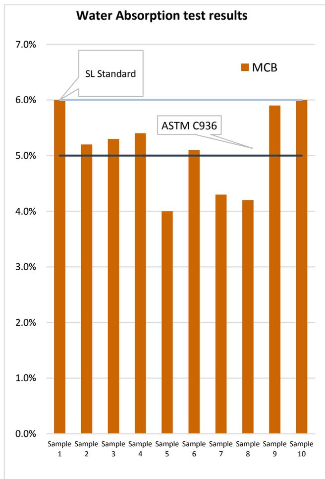
Figure 19: Cold-water absorption test results.
