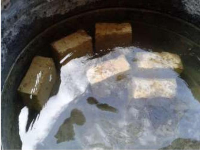
Figure 5: Measuring cold-water absorption
