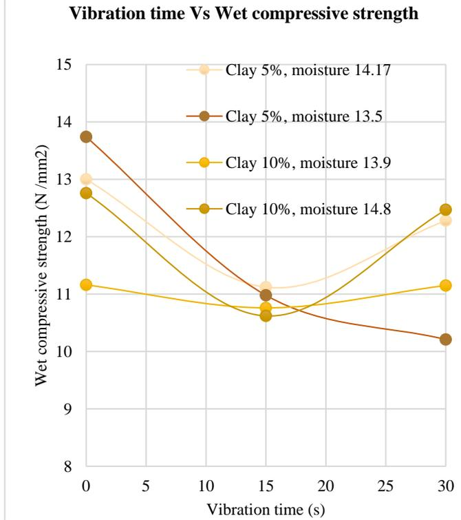
Figure 13: Variation of wet compressive strength with vibration time.
