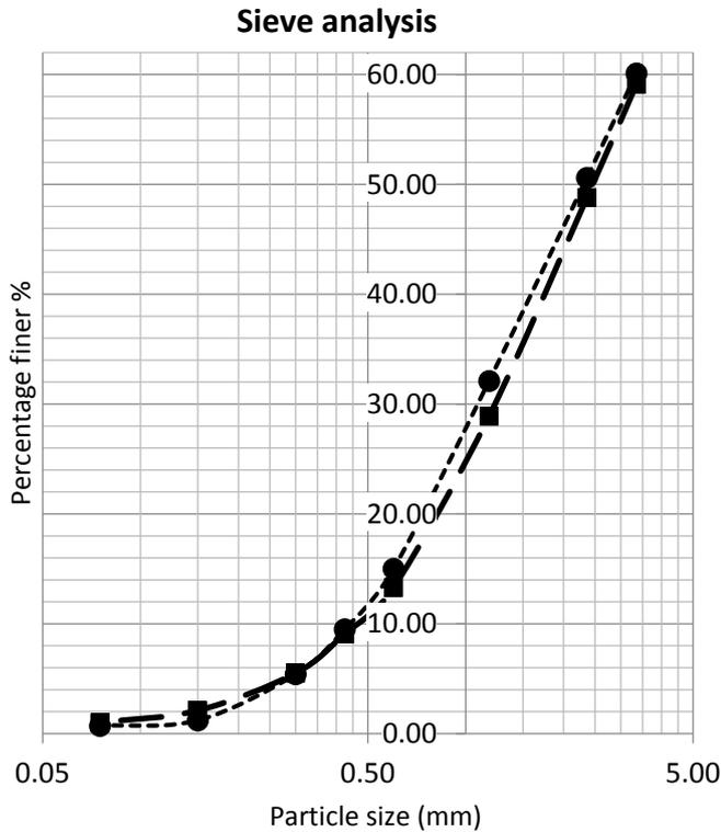
Figure 8: Particle size distribution of soil used for Mud concrete Paving Blocks
