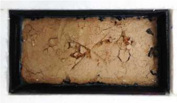
Figure 20: surface of the test specimen after the freeze-thaw cycle test
