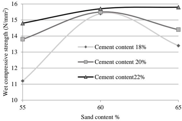
Figure 14: The behavior of wet compressive strength with cement content.
