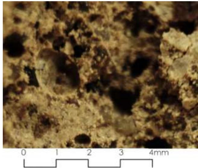
Figure 18: Microscopic image of pores structure of mud paving block.
