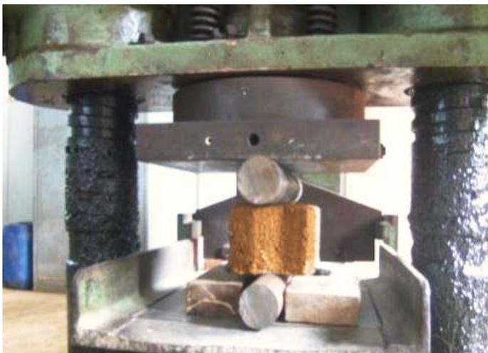
Figure 4: Measuring tensile splitting strength of mud concrete paving block
