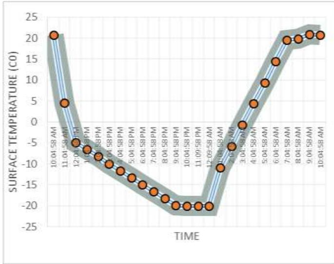
Figure 6: Time- temperature cycle for freeze thaw test
