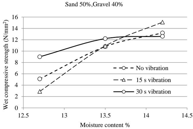
Figure 10: Variation of wet com. strength with sand 50% and gravel 40%
