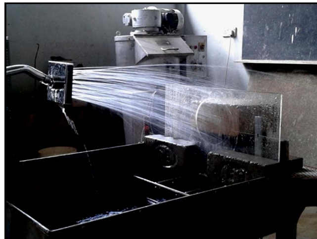
Fig. 15. Accelerated erosion test conducted in laboratory.
