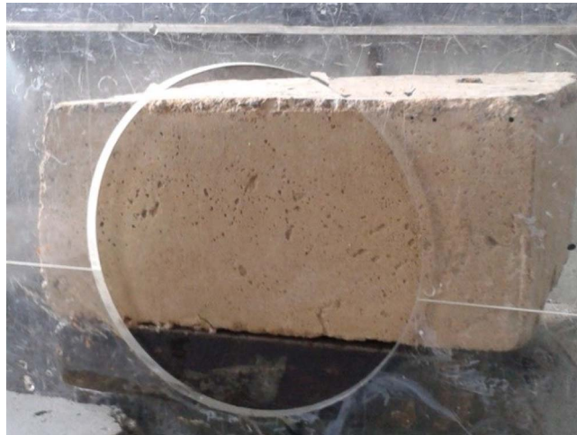
Fig. 16. The surface of MCB before carrying out the accelerated erosion test.
