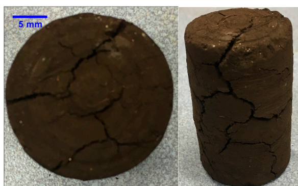
Figure 1. Fractures after low-temperature drying.
