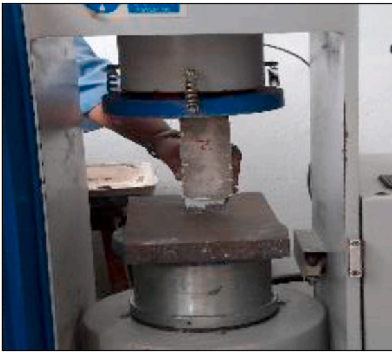
Fig. 7. Conducting lap shear strength test using compressive strength testing machine.
