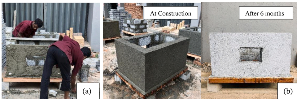
Fig. 9. a) Development of model house units b) House units after 6 months.
