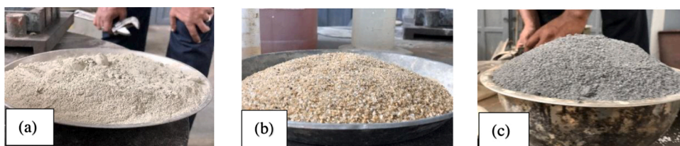
Fig. 4. Materials - a) Cement b) Sand c) Bottom ash.
