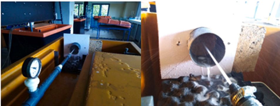
Fig. 3. Accelerated erosion test procedure.
