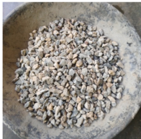
Fig. 5. Crushed construction waste.
