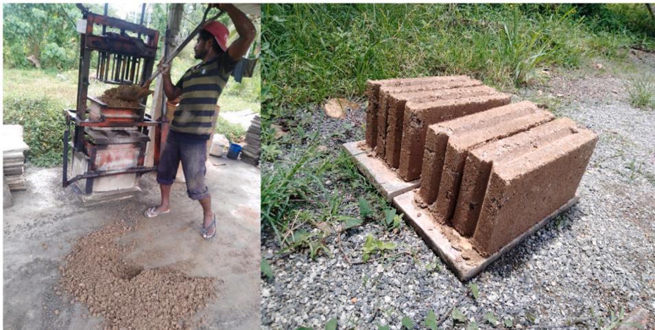
Fig. 8. Industrial scale block making process.
