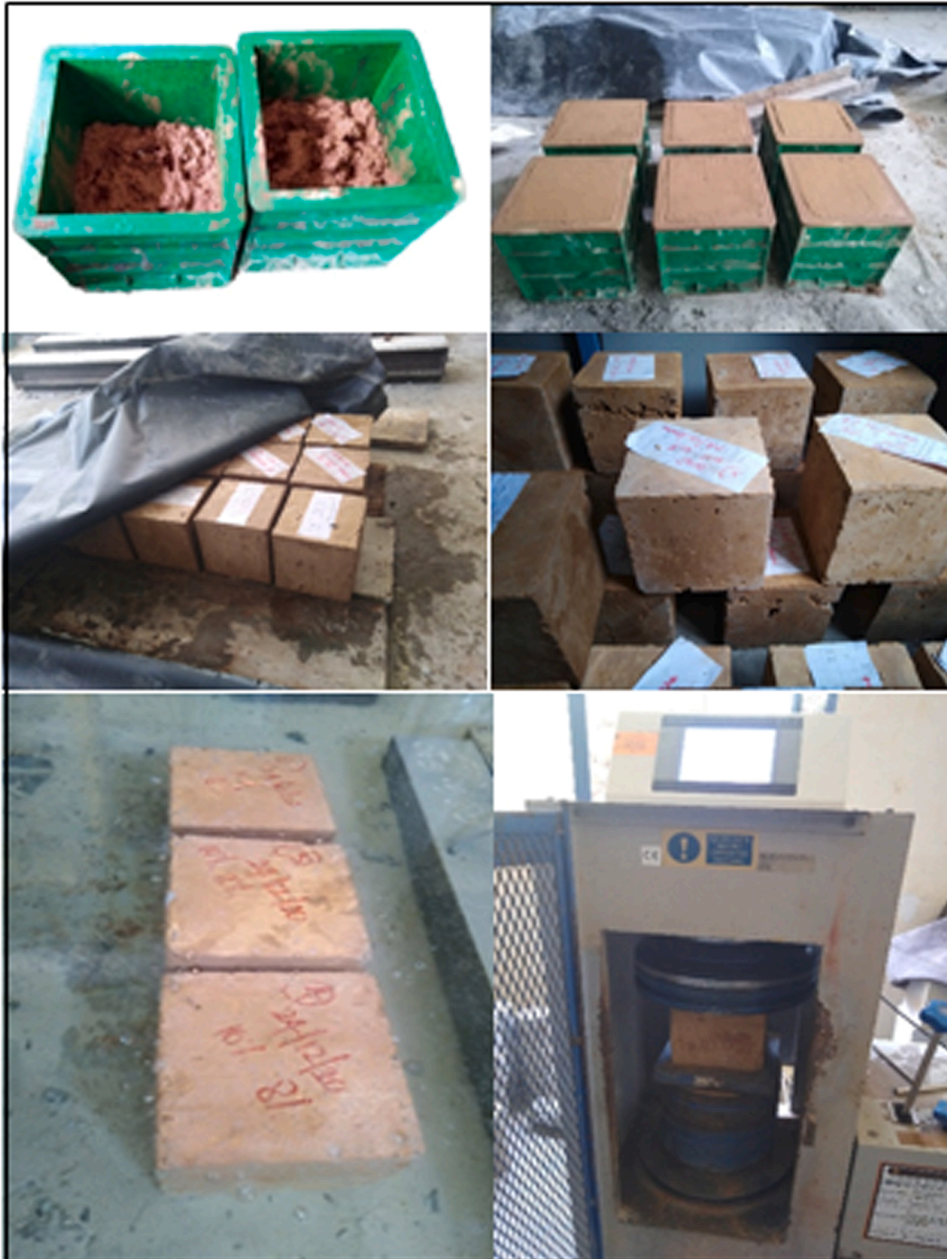
Fig. 2. Block casting and compressive test procedure.
