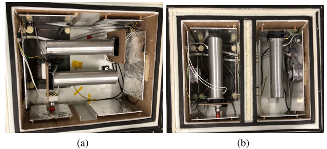
FIGURE 8. Test set ups used to determine calorimeter conduction heat leakage (a) through outside walls only; (b) when operated as two chambers.
