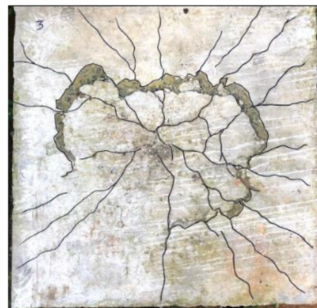
Fig. 2. Crack pattern on the tension face of heavily damaged specimens.
