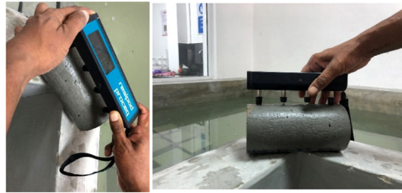
Fig. 5 Proceq's Resipod meter measuring resistivity
