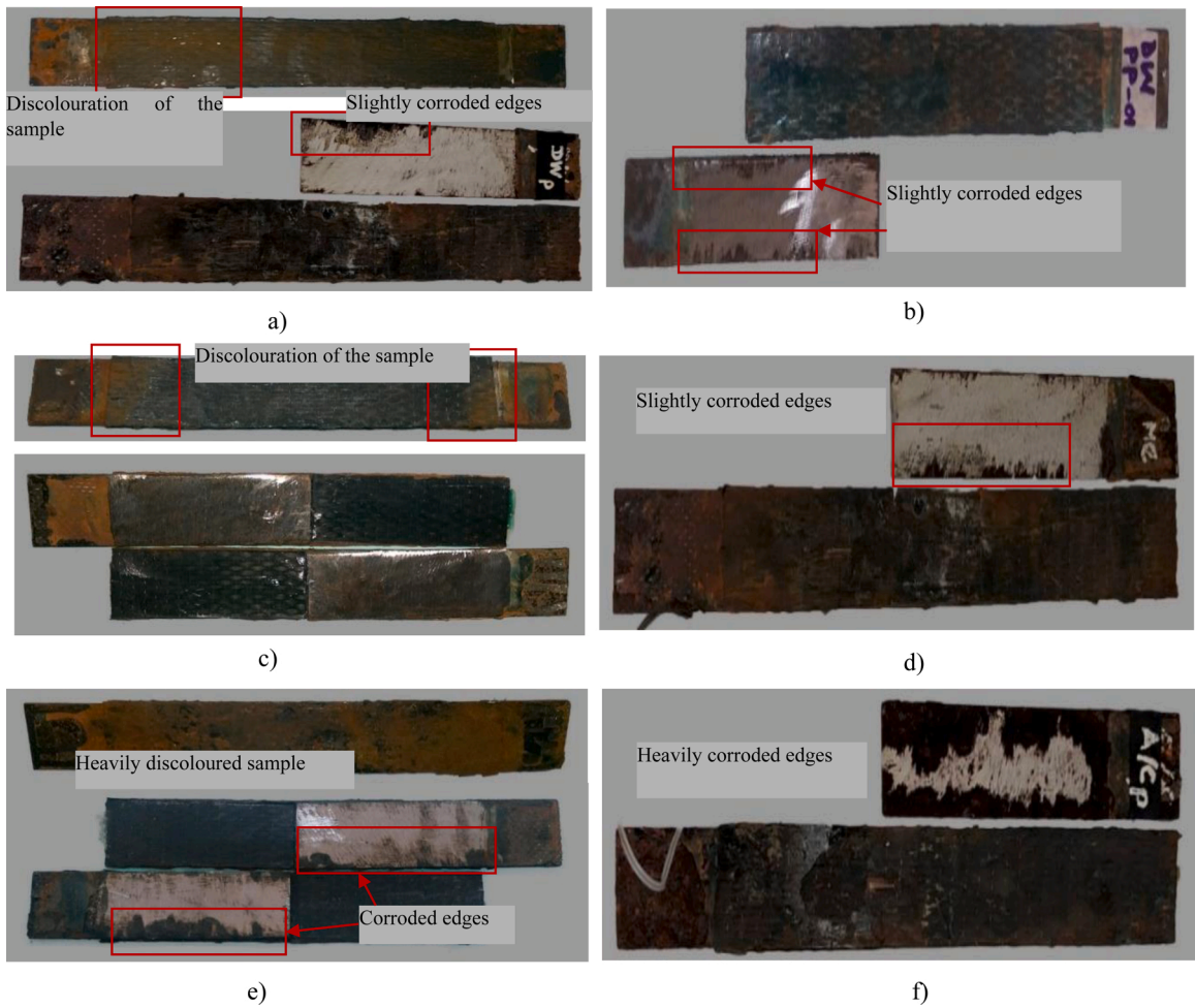
Fig. 5. Failure modes of the specimens: a) Distilled water at ambient temperature (Ave. 28 °C)/Conditioning period - 6 months b) Distilled water at ambient temperature (Ave. 28 °C)/Conditioning period - 12 months c) Simulated seawater (5% NaCl) at ambient temperature/Conditioning period – 6 months d) Simulated seawater (5% NaCl) at ambient temperature/ Conditioning period - 12 months e) Dry /wet cyclic condition in simulated seawater – 5% NaCl at ambient temperature/ Conditioning period - 6 months f) Dry /wet cyclic condition in simulated seawater – 5% NaCl at ambient temperature/ Conditioning period - 12 months.
