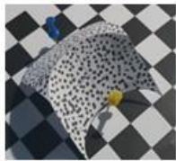
3D Reconstructed Miura Ori curved crease fold mesh by using LiDAR scanning
