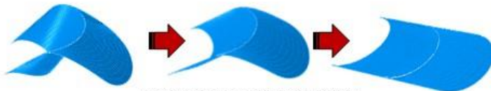
Stages in numerical simulation - Fully folded to intermediate stage to final deployment
