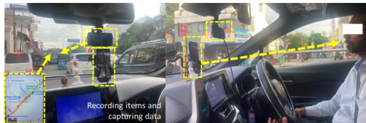
Figure 2. Experimental setup: driver facial expression recording, road scenario recording, navigation of the test
