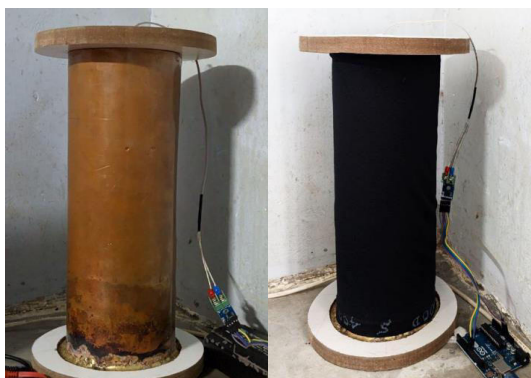
Figure 2_ Bare and test subject wrapped copper Cylinder with lids and the thermocouple equipped.
