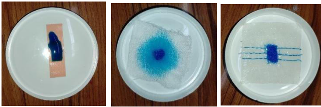
Fig 3: Represented here are (a) Dettol plaster (Varun Medimpex Inc., India) (b) Conventional cotton gauze ((Suntex Industries (Pvt) Ltd, Sri Lanka) (c) Developed wound dressing with thread based microfluidic platform
