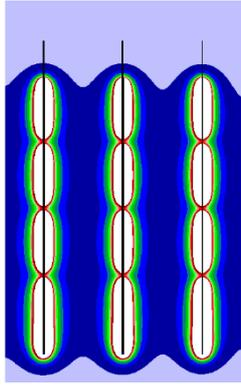
Figure 9: Vertical explosive energy distribution for four charging decks pattern
