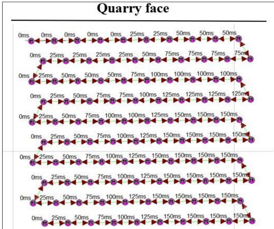
Figure 2: Downhole delay pattern with delay time for existing blast simulation
