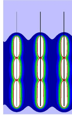
Figure 12: Vertical explosive energy distribution for three charging decks pattern
