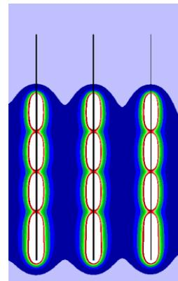
Figure 13: Vertical explosive energy distribution for four charging decks pattern
