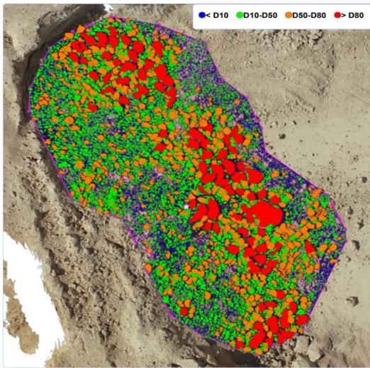
Figure 15: Muck pile area analysis for the test blast
