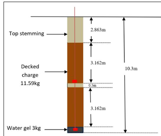
Figure 4: Two-deck charging pattern of holes - ANFO quantity per hole is reduced
