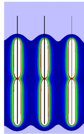
Figure 7: Vertical explosive energy distribution for two charging decks pattern
