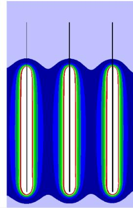
Figure 6: Vertical explosive energy distribution for single deck charging pattern
