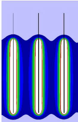
Figure 10: Vertical explosive energy distribution for single charging deck pattern
