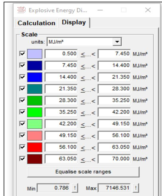
Figure 14: Scale range of static vertical energy distribution of explosive charge for the optimised blast
