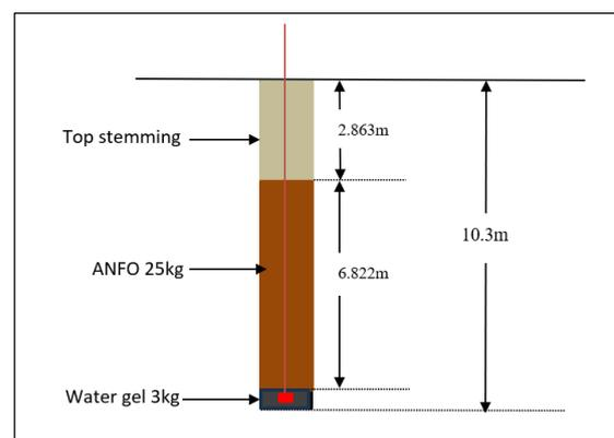
Figure 1: Existing charging pattern of blast holes
