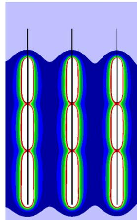
Figure 8: Vertical explosive energy distribution for three charging decks pattern
