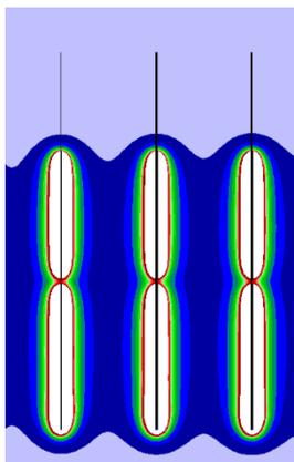
Figure 11: Vertical explosive energy distribution for two charging decks pattern
