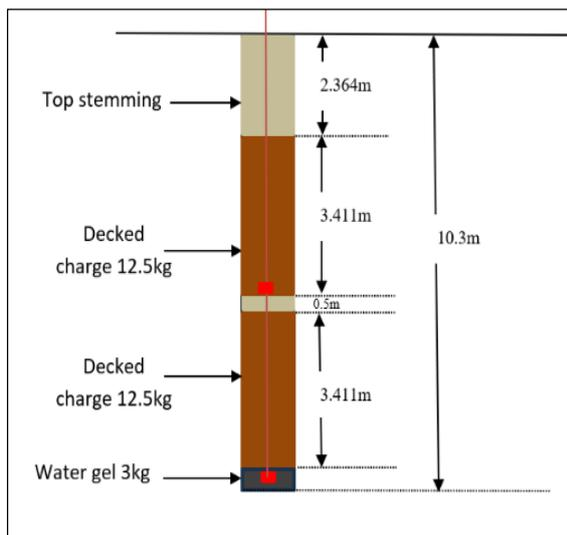
Figure 3: Two-deck charging pattern of holes - ANFO quantity per hole is kept constant
