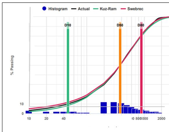
Figure 16: Fragmentation analysis for the test blast
