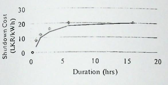
Figure 9 : Variation of Shutdown Cost versus Duration
