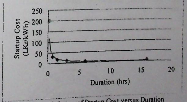
Figure 7 : Variation of Startup Cost versus Duration
