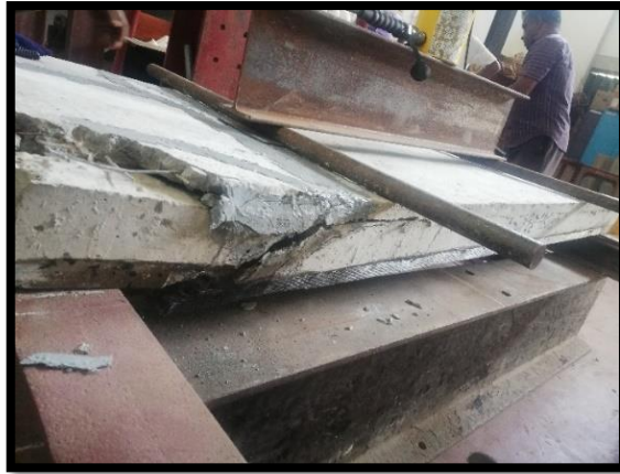
Figure 5.9: Loosening of strength between in-situ concrete and pre-stressed beam.
