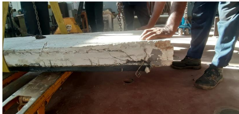
Figure 5.13: Shear and flexural cracking on strengthened models with FRP.
