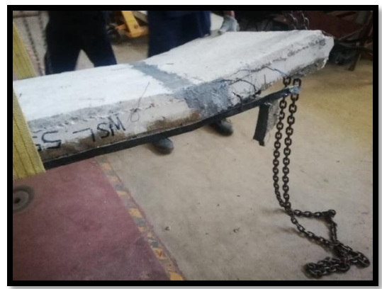
Figure 5.7: Shear cracks near CFRP wrappings
