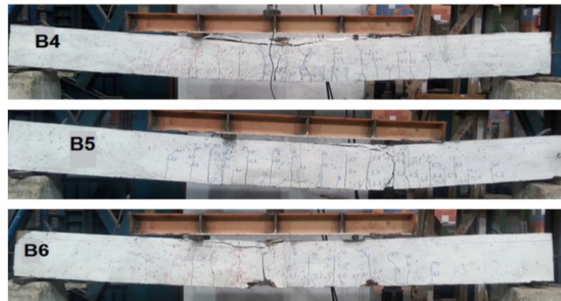
Figure 2.27: Crack pattern at the controlled specimens
