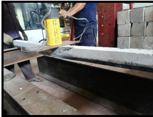
Figure 5.10: Pre-stressed beams failed due to crushing and propagation of flexural cracks.
