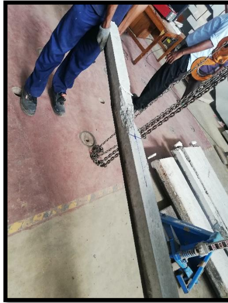
Figure 5.14: Strengthened Pre-stressed beams failed due to crushing & propagation of flexural cracks.
