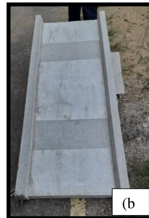
Figure 4.9: Surface preparation (a) Grinding off weak layer of concrete (b) Appearance of ground concrete surface.
