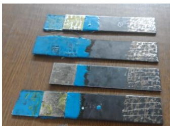
Figure 5: Normal Modulus CFRP Failure Mode (Delaminate /Interface Debonding)
