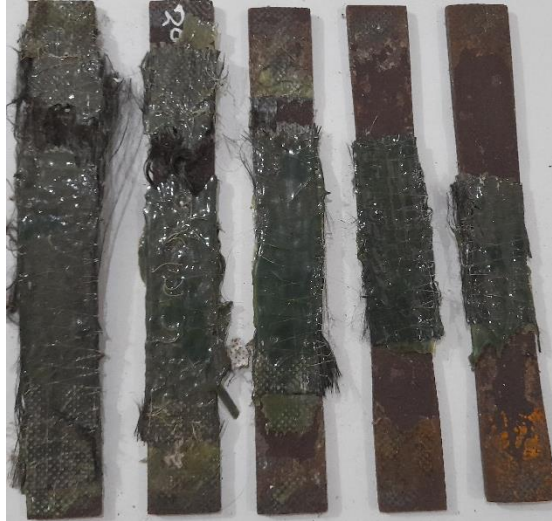
Figure 4-59: Failure mode of steel member without CSH variation with bond length
