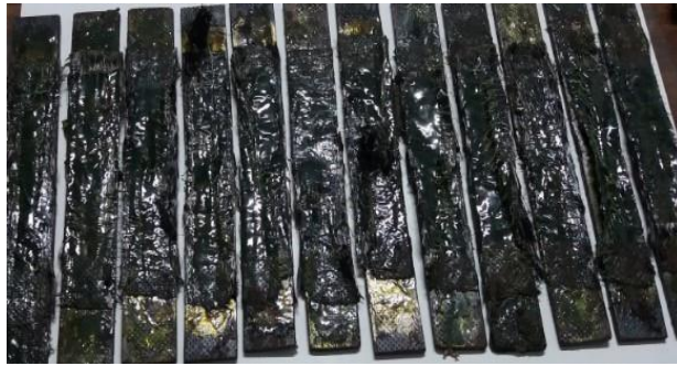
Figure 4-28: Failure mode of non-conditioned CFRP strengthened specimen
