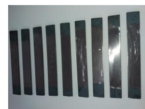
Figure 3 :Primer coted steel plate
