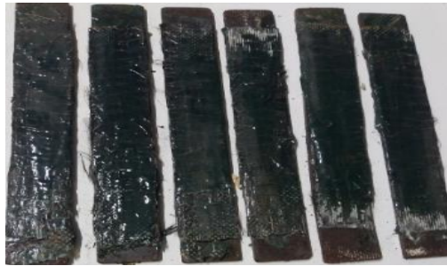
Figure 4-45: Failure mode of CFRP strengthened offset CSH
