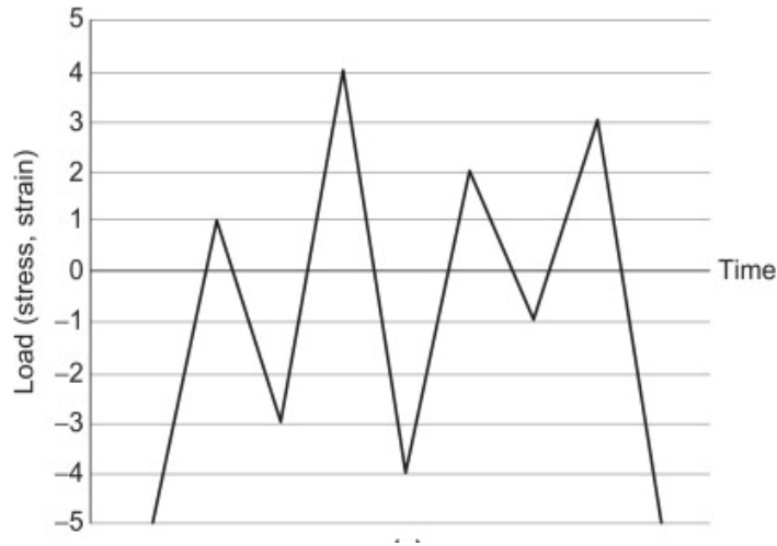
Figure 2-7: Stress variations with time linked to variable amplitude loads
