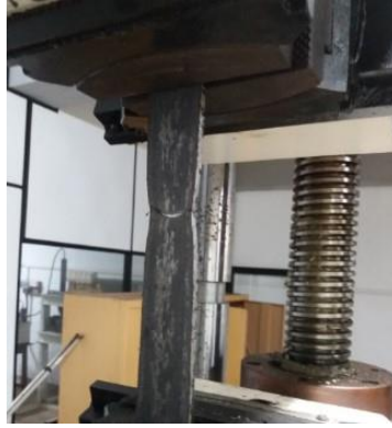
Figure 4-11: Failure mode of plane specimens non-strengthened plates without CSH
