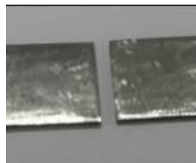
Fig 2(a): Grinded Surface
