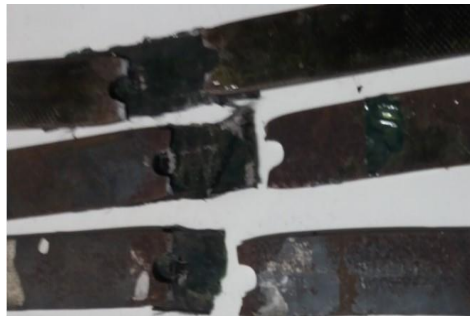
Figure 4-56: Failure mode of CSH due to bond length variation
