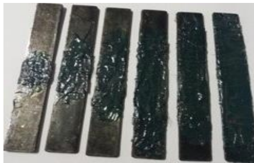
Figure 4-54: Schematic view of the CFRP strengthened specimen with different bond length (Scale 1:2) (a) elevation (b) Plane view (c) typical specimen
