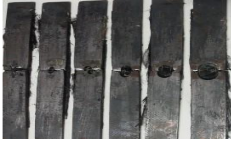
Figure 4-34: Failure mode of conditioned CFRP strengthened CSH
