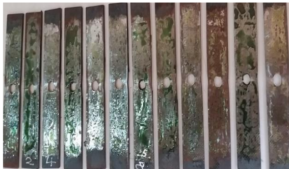
Figure 4-14: Failure mode of plane specimens non-strengthened plates with the CSH
