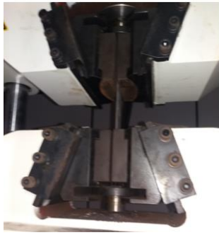
Figure 7 :Test setup to apply tensileload
