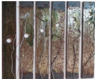
Figure 4-49: Typical specimen of non-strengthened strain gauge attached offset CSH
