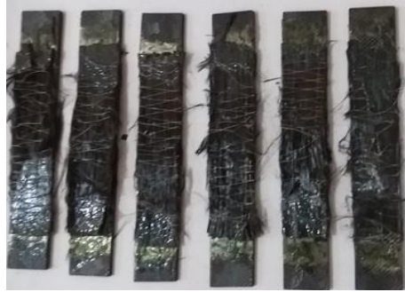
Figure 4-17: Failure mode of CFRP strengthened plane specimens without CSH
