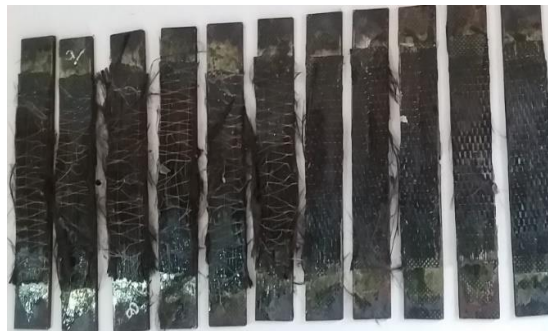
Figure 4-20: Failure mode of CFRP-strengthened steel element with CSH
