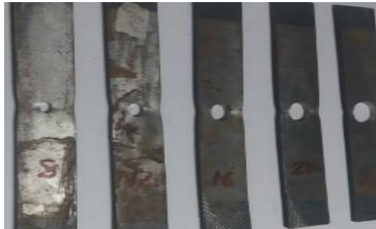
Figure 4-25: Failure mode of non-conditioned non-strengthened CSH
