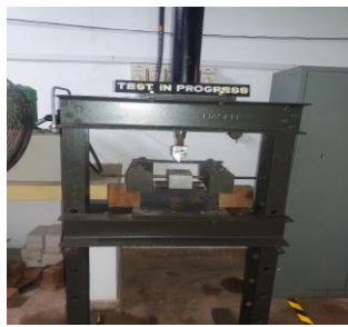
Figure 5:Test setup to apply cyclic flexure load
