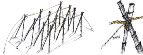
Fig. 12: Tanaway Stand: it has straight ropes without sagging, tie end to end on the cross of Bamboos Source: author
