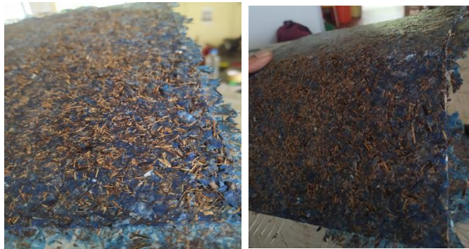
Figure 28: Prepared composite boards with improper bonding
