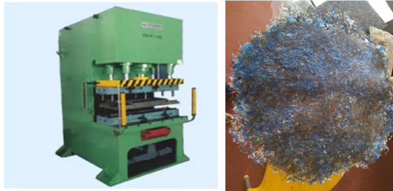
Figure 10: Hot Press Machine and Prepared Laminated Sheets
