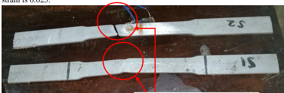
Failure points of steel coupons
