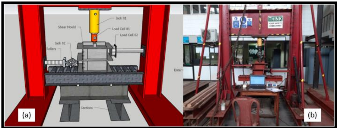
Figure 6.4: Large-scaled direct shear testing setup (a) proposed setup and (b) developed setup
