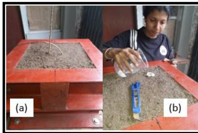
Figure 6.12: Sample installation (a) sensor installation, (b) sand pile installation
