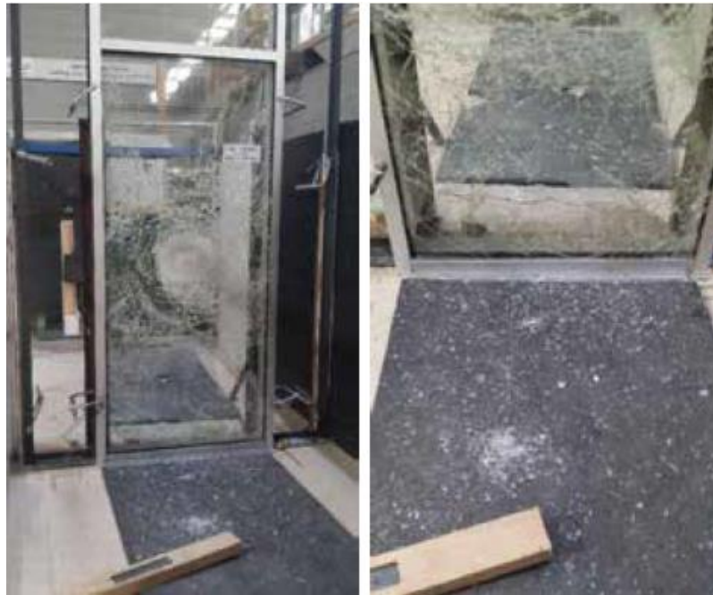
Figure 2.21 - Tested window panel (Mejorin et al., 2019)
