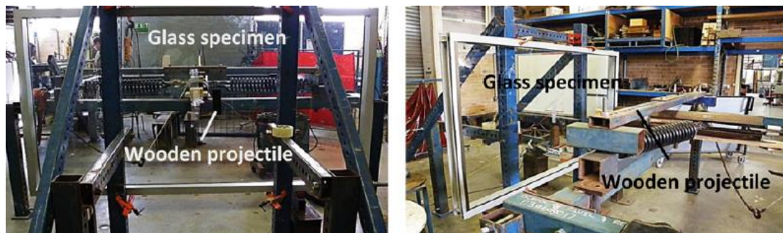
Figure 2.26 - Impact testing apparatus with a two-spring catapult system (Zhang et al., 2013)
