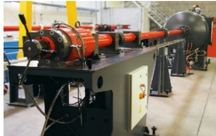
Figure 5.1 Single-stage gas gun
