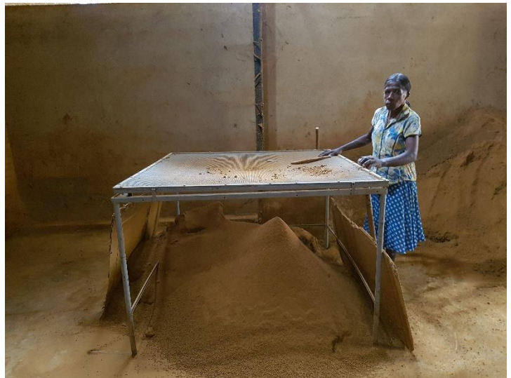
Figure 3.26; Crushed sludge sieving
