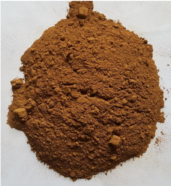
Figure 3.7; Sludge Powder (Particle size < 0.6mm)
