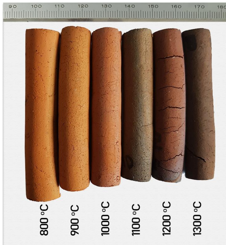
Figure 3.18; Sintered sludge cylinders for different temperatures
