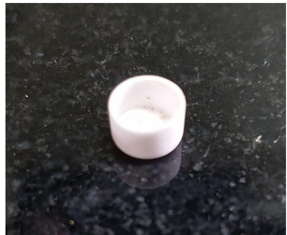
Figure 3.5; 20mg sludge Holder for TGA testing
