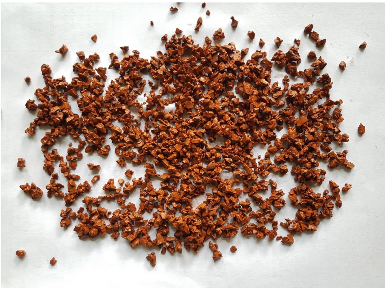
Figure 3.19; Water saturated fine aggregates for water absorption test
