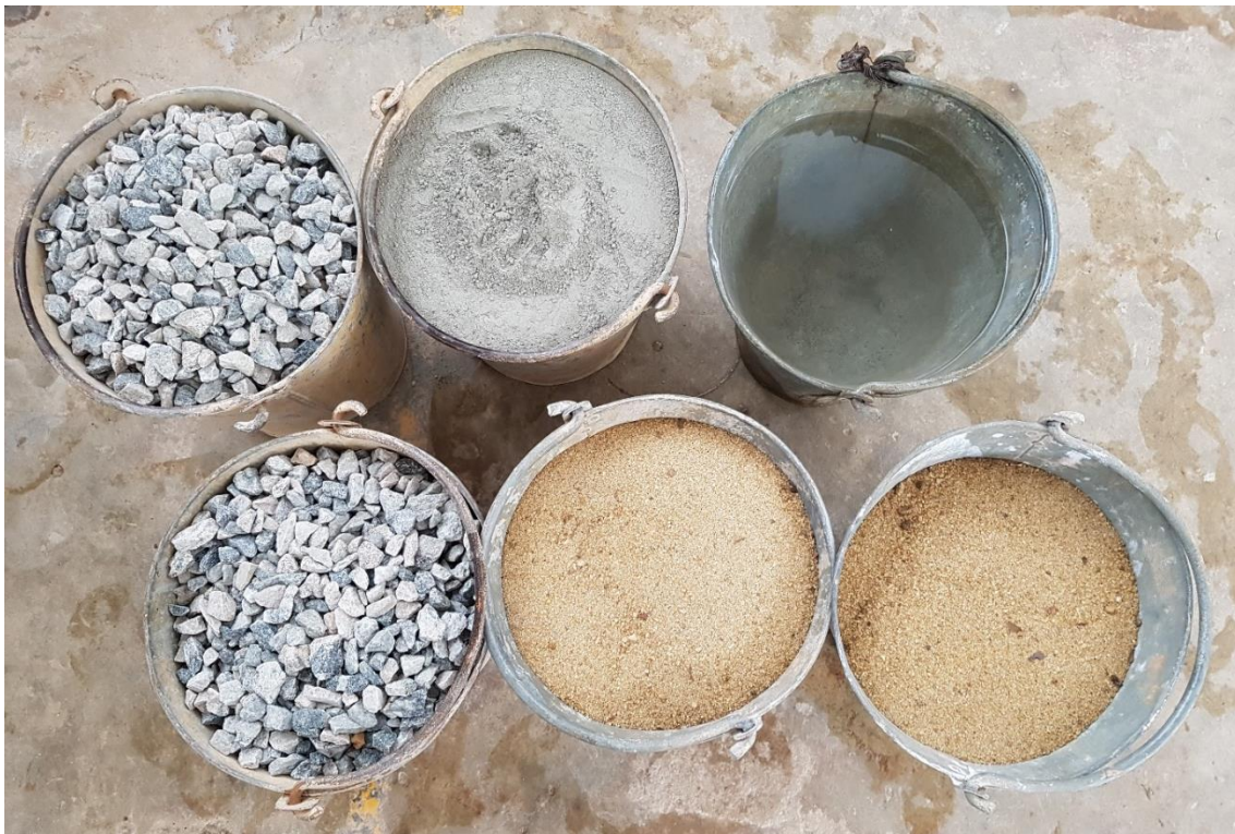
Figure 3.33; Raw materials to cast concrete
