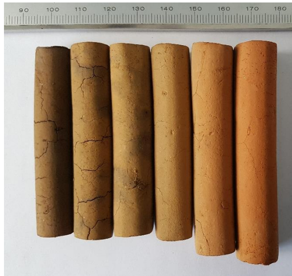
Figure 3.14; Sintered sludge cylinders for 800°C to 1300°C temperatures
