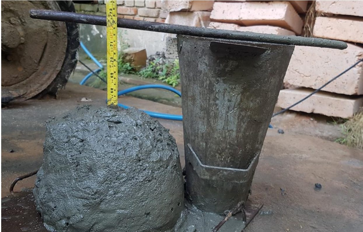
Figure 3.36; Measuring the slump
