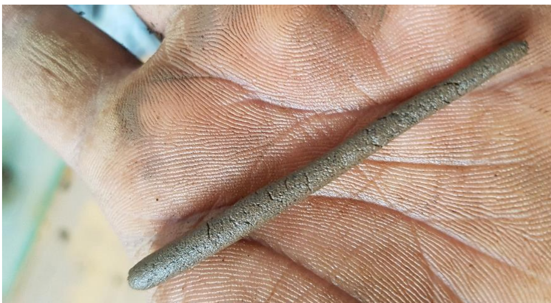
Figure 3.3; 3mm sludge thread for plastic limit test
