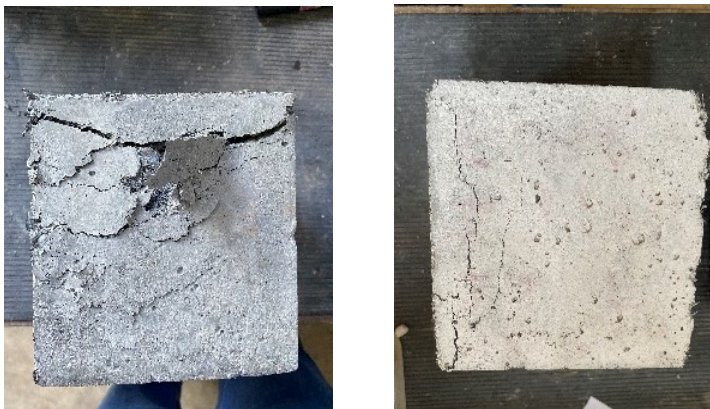
Figure 3.6. Observed failure pattern of Series 2 and Series 3 specimens
