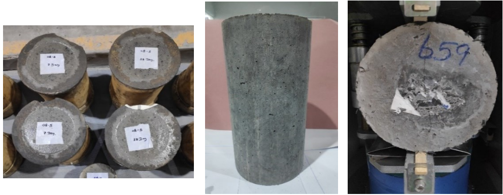
Figure 6.3. Preparation and testing of splitting tensile cylinders
