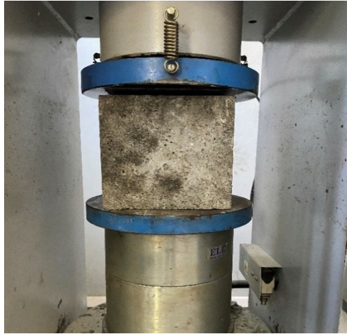
Figure 3.3. General view of the instrumental setup of compressive strength testing of sample specimen
