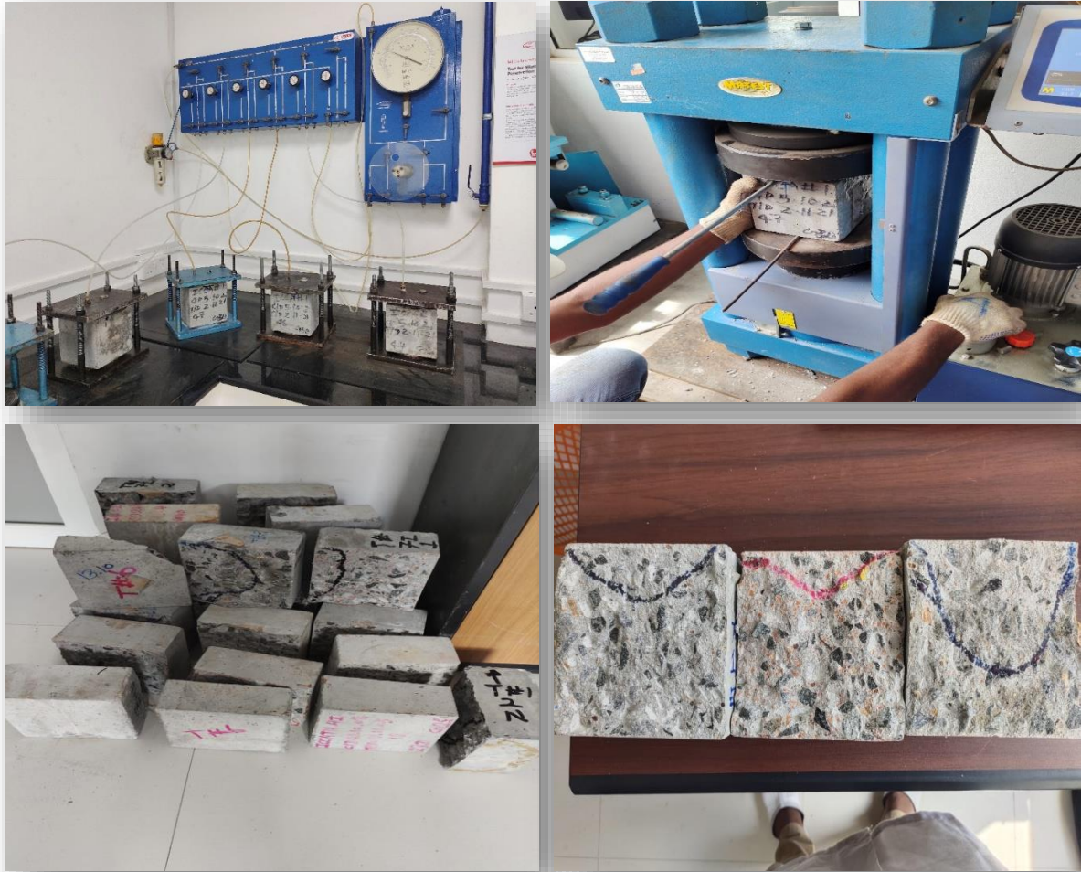
Figure 3-16: Water permeability test.
