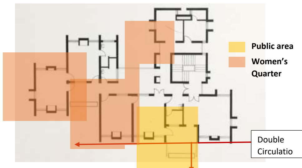
Figure 08: Plan of EPUET Faculty Housing highlighting separate women's quarter and double circulation system.
