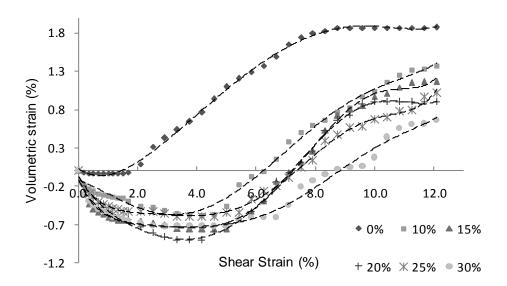
Figure 3: Typical plot of variation of volumetric strain with shear strain for 5.6 mm crumb size with different percentage of rubber mix at normal stress of 100 kN/m<sup>2</sup>
