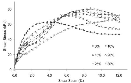
Figure 2: Typical plot of variation of shear stress with shear strain for 5.6 mm crumb size with different percentage of rubber mix at normal stress of 100 kN/m<sup>2</sup>
