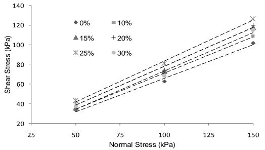
Figure 4: Typical plot of variation of shear stress with normal stress for 5.6 mm crumb size with different percentage of rubber mix
