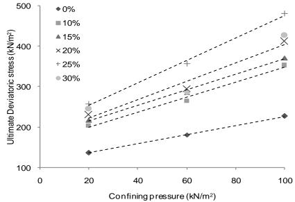
Figure 8: Effect of 5.60 mm rubber on ultimate deviatoric stress for different composition
