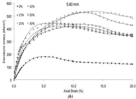
Figure 6: Stress-strain curves for confining pressure of 100kN/m<sup>2</sup> for different rubber size: (a) 1.00 mm, (b) 5.60 mm
