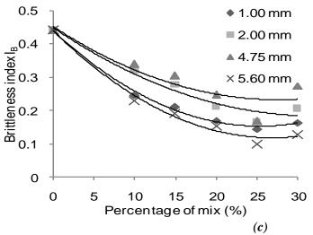
Figure 9: Typical plot of variation of brittleness index of sand with inclusion of rubber for confining pressure of 100 kN/m<sup>2</sup>
