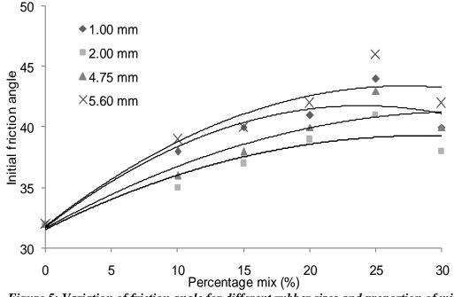
Figure 5: Variation of friction angle for different rubber sizes and proportion of mix
