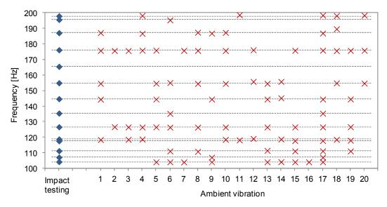
Figure 5 Natural frequencies identified by impact testing and 20 ambient vibration records
