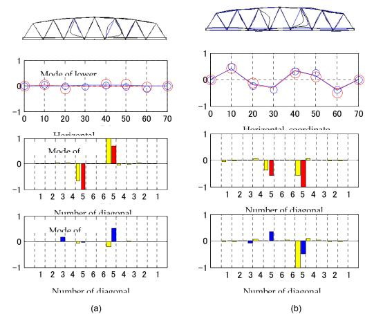
Figure 6 Modal amplitudes corresponding to (a) local mode at 9.264 Hz and (b) coupled mode at 9.325 Hz. The vi-bration modes identified experimentally are compared with those obtained theoretically.
