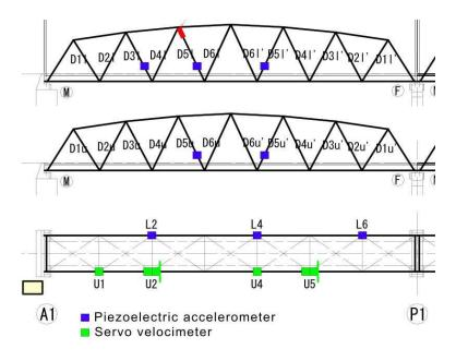
Figure 3 Positions of accelerometers in Measurement 3
