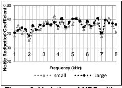
Figure 6: Variation of NRC with particle size
