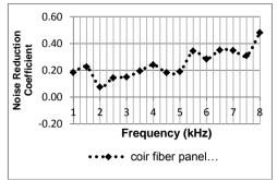
Figure 7: NRC of Coconut coir fiber panel
