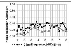
Figure 5: Variation of NRC with tile thickness
