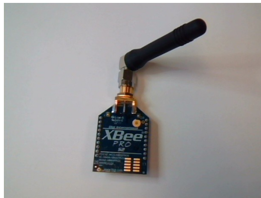
Figure 2. RF transmission module
