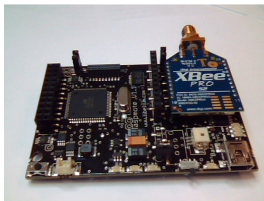
Figure 3. Sensor control module with RF transmission module plugged onto it.
