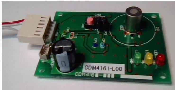
Figure 5. The Carbon Dioxide sensor module
