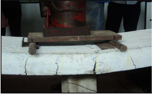
Figure 12: Crack propagation of R6-CS1
