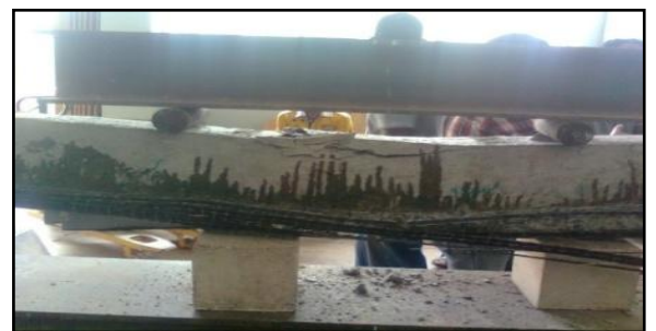
Figure 18: Debonding failure of FRP strengthened beam
