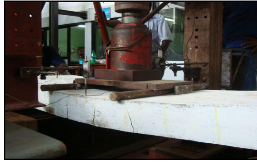
Figure 13: Crack propagation T10-CS1
