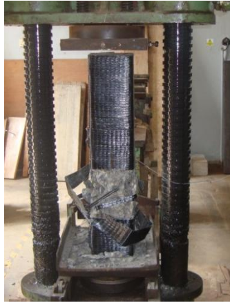
Figure 8 – Failure mode of CFRP confined column specimens C4 and C5
