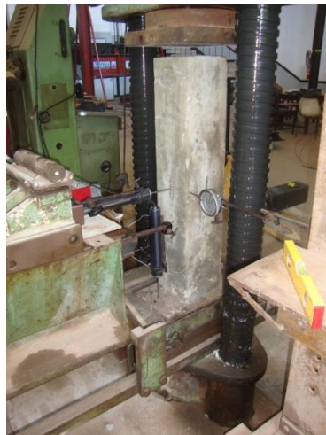
Figure 5: LVDT and Dial gauge arrangement
