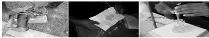
Figure 6: Total and free chloride ion concentration measurement procedure (a) Concrete powder collecting (b) Sieved concrete powder (c) Titration against \text{AgNO}_3
