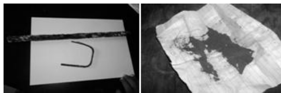
Figure 7: Rust production measurement procedure (a) Bars were removed from beams, (b) Scraped rust
