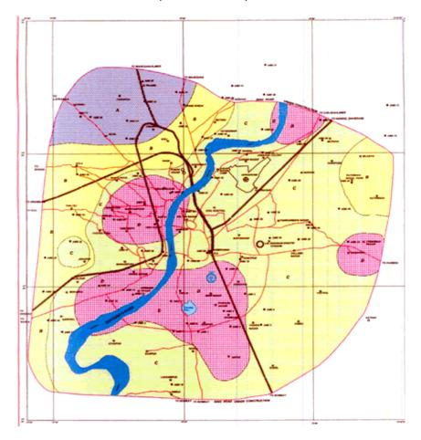
Figure 2. Preliminary seismic hazard map, 1<sup>st</sup> level of Microzonation of Ahmedabad city
