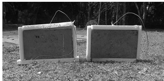
Figure 6 – Cover the blocks using insulators
